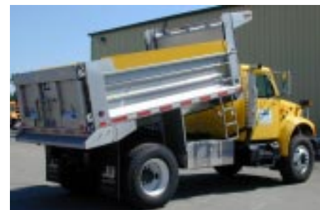
11 foot aluminum crossmemberless dump body on a 2001 International 4900.
