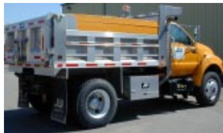
10 foot aluminum dump body on a 2000 Ford F750.
