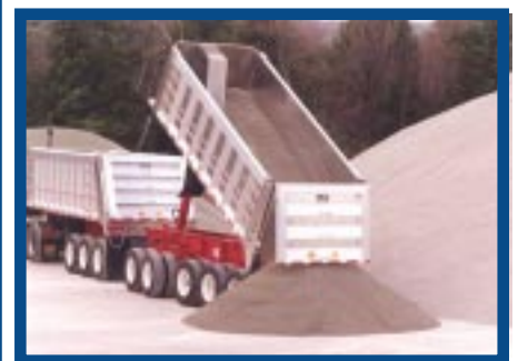
DynaHauler/FTA-D, steel frame/aluminum body double dump trailer
