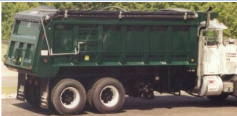
DynaHauler/LWC, lightweight crossmemberless dump truck body
