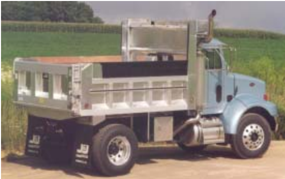
This size dump body is ideal for a medium-duty chassis. Lengths from 9 to 12 feet.
