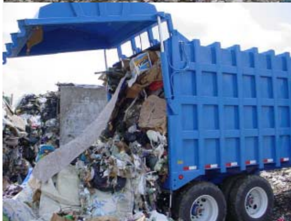
This trailer is completely self-contained and powered by a Duetz diesel power unit. It is used for packing and discharge of municipal solid waste.
