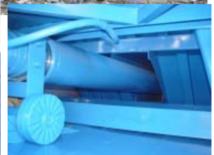
The cylinder on this unit is 9" in diameter with a first stage 89,000 lb. force capability at 1300 psi.
