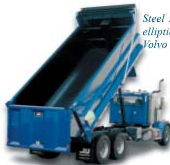
Aluminum semi elliptical on a International chassis
